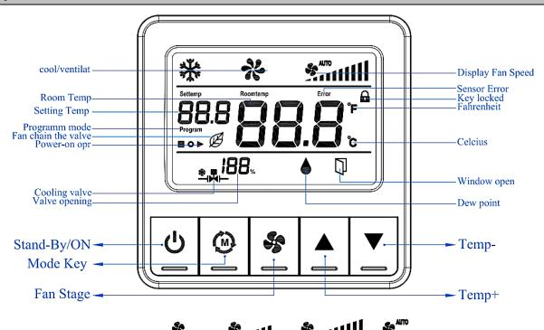
Display Fan Speed: Fan Low Fan Medium Fan High Fan Auto
